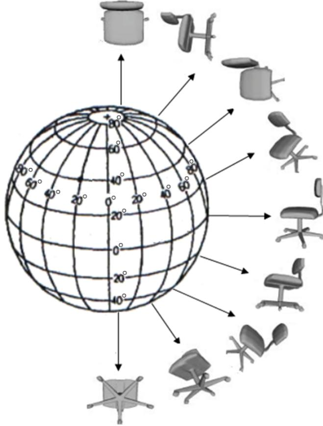
FIGURE 2. The sphere algorithm of 3D model projection views
