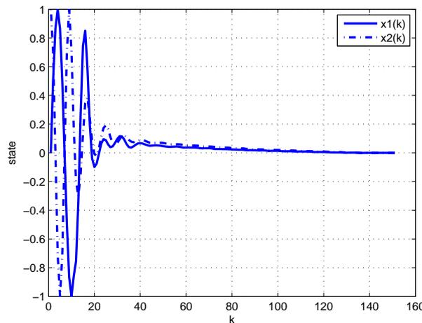
FIGURE 1. State trajectories of the system with quantization and overflow nonlinearities considered in Example 4.2
