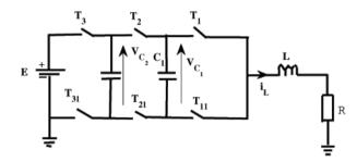
FIGURE 1. Multicellular converter
