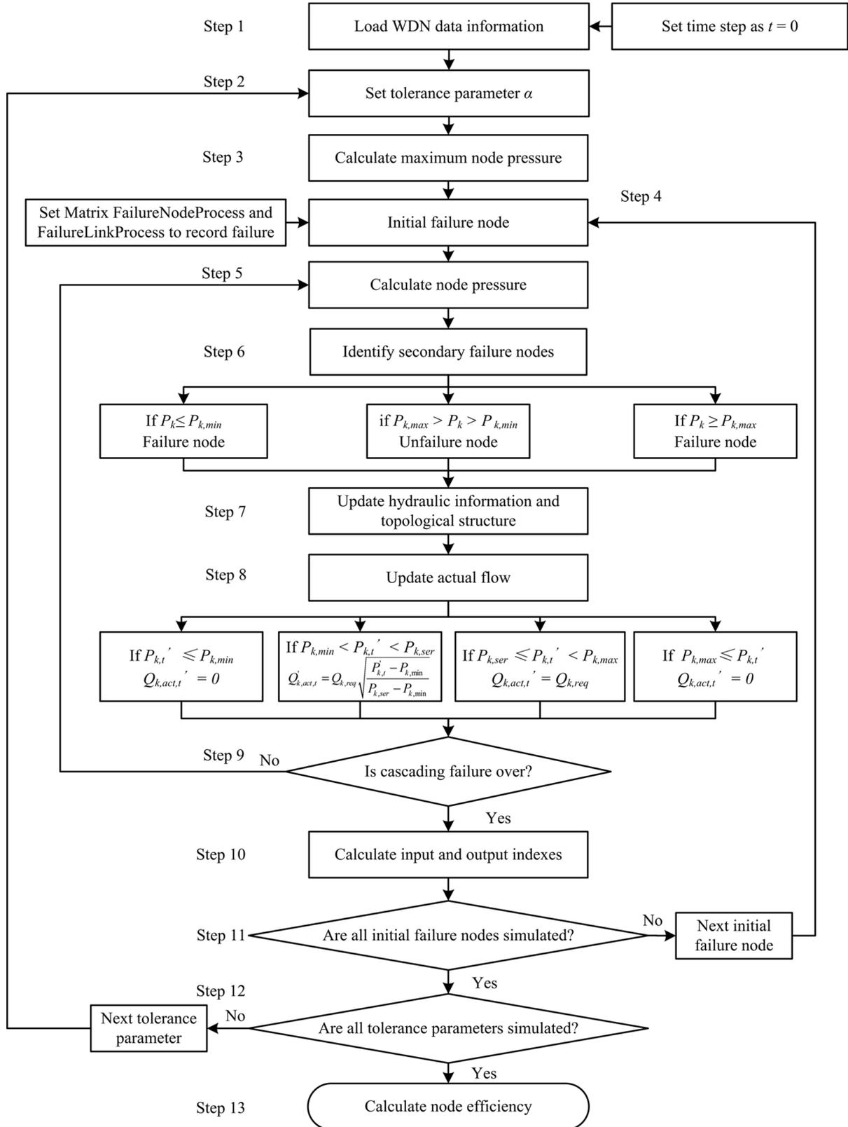
FIGURE 1. Simulation process flowchart of cascading failures in WDN based on DEA
