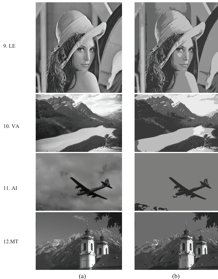
FIGURE 7. The final image segmentation results: a) the original image; b) the image segmentation results based on the IKM method
