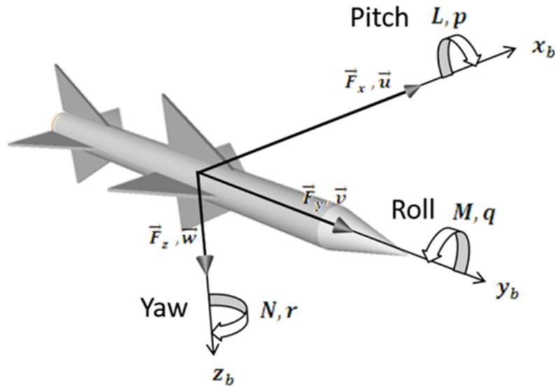
FIGURE 2. The illustration of pitch, yaw, and roll
