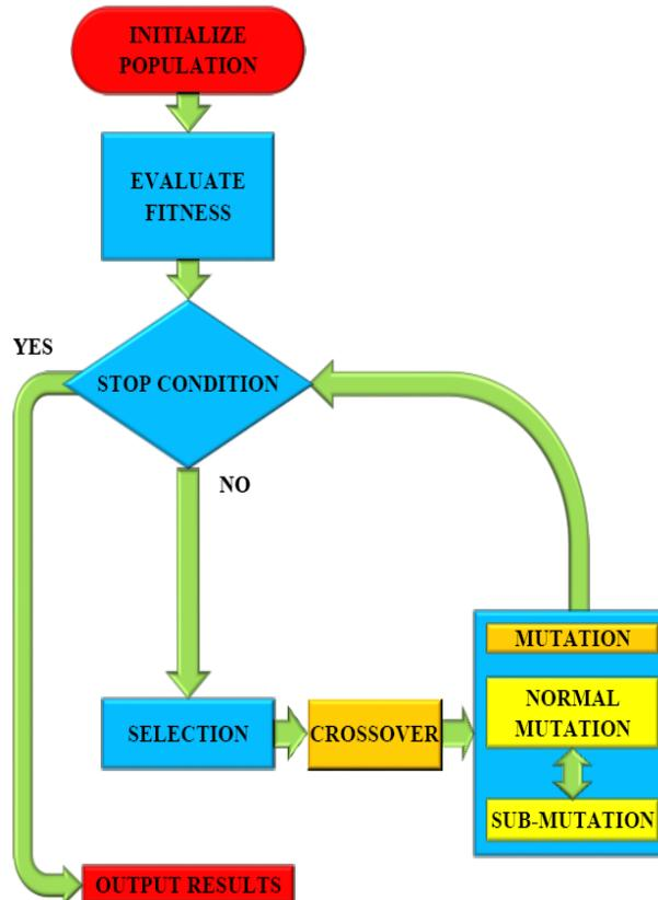
FIGURE 6. The flowchart of modified sub-genetic algorithm
