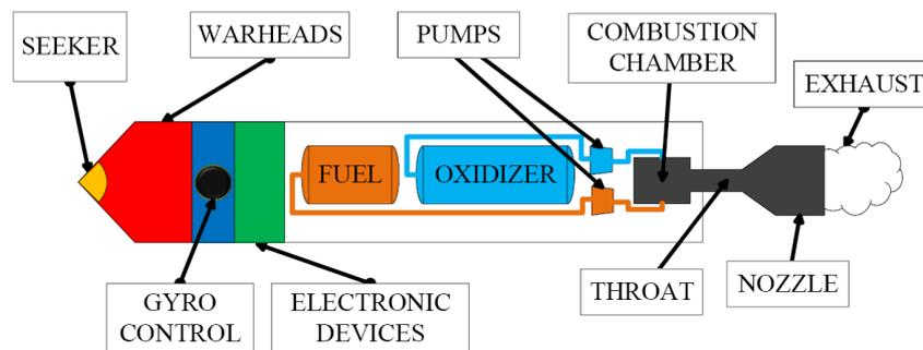
FIGURE 1. The parts of liquid rocket engine
