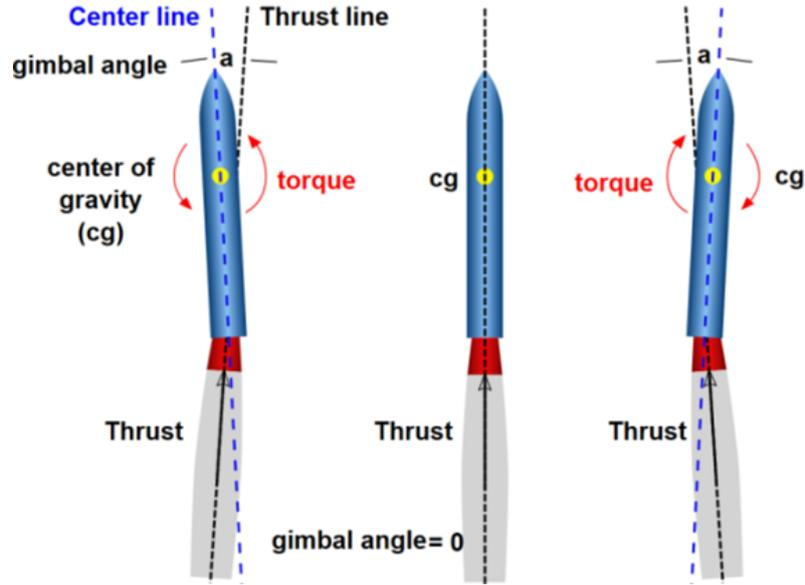
FIGURE 3. Representing of nozzle angle, gimballed angle, and other parameters
