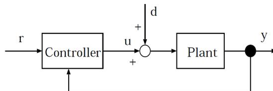
FIGURE 1. Block diagram of a PID control system
