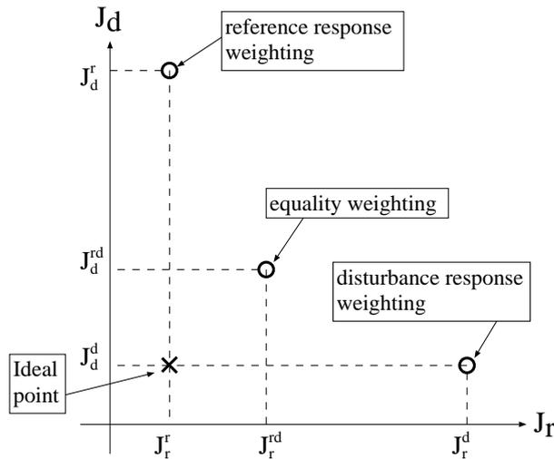
FIGURE 2. Servo/regulation and equality weighting optimization [9]
