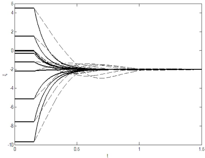
FIGURE 8. Comparison of the convergence rate in Example 4.3 for deformed protocol (8) with  $q = 0.2$  with maximum tolerable uniform delay communication in linear protocol (dashed lines), and the protocol (2) with no delay (solid lines)
