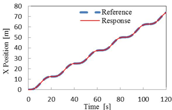
FIGURE 3. Tracking performance of the  $x$  position
