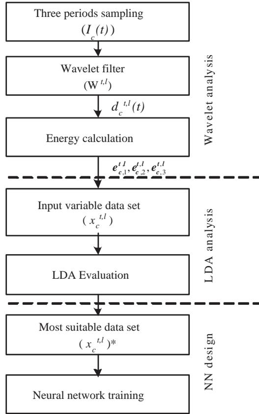
FIGURE 5. Flowchart of designing detection system
