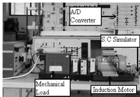
FIGURE 8. Laboratory experimental setup
