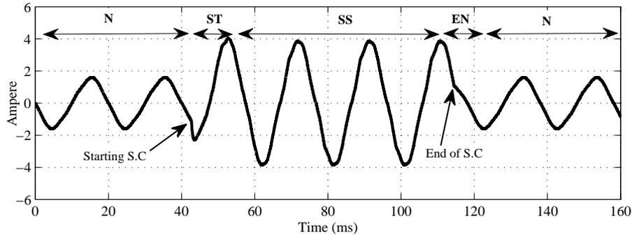
FIGURE 2. Temporary short circuit fault
