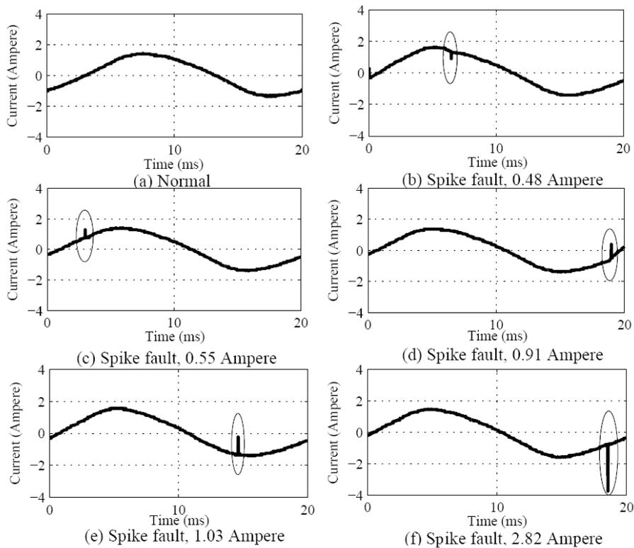
FIGURE 1. Spike short circuit fault
