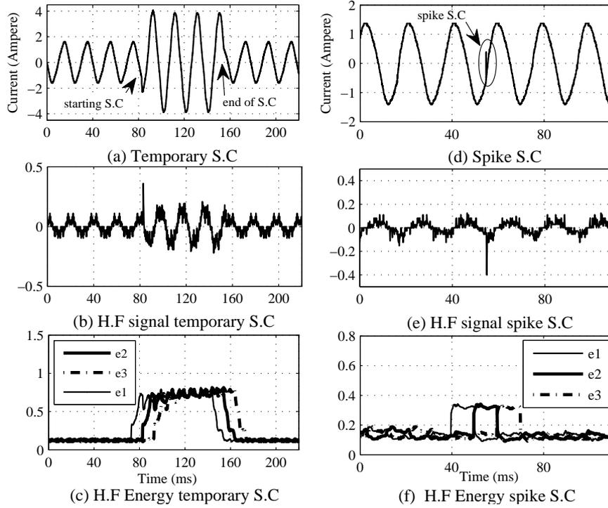
FIGURE 6. Current signal treatment using wavelet transform
