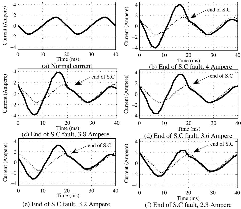
FIGURE 4. End of short circuit
