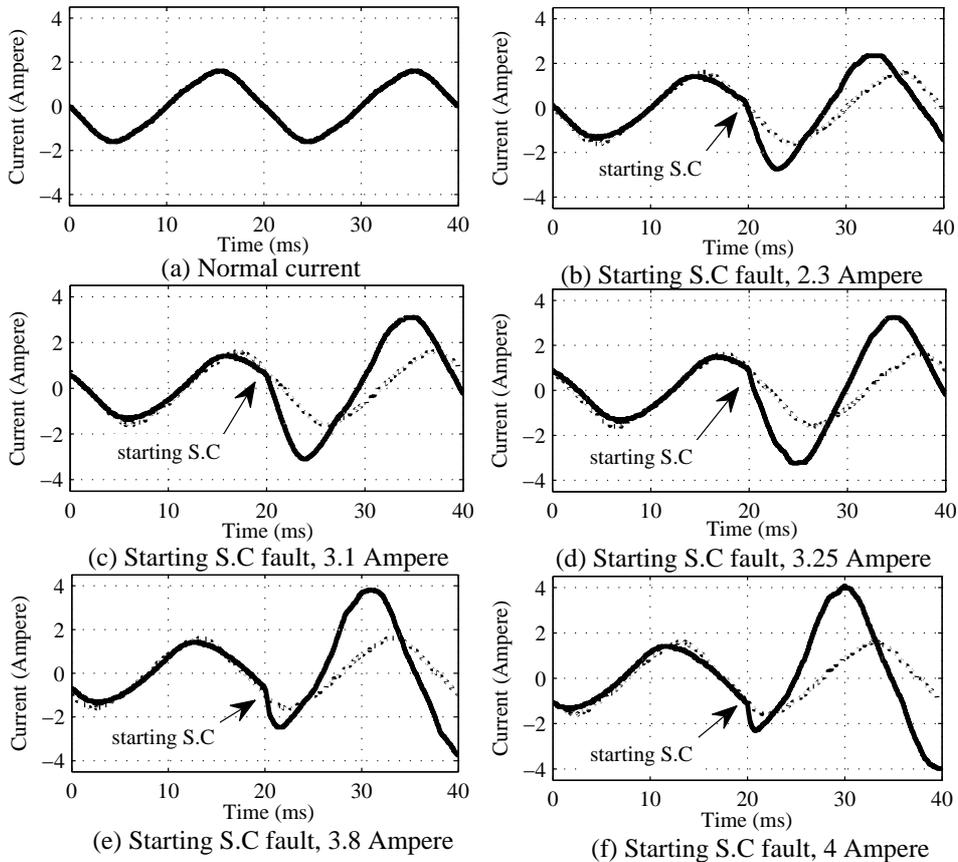
FIGURE 3. Starting short circuit
