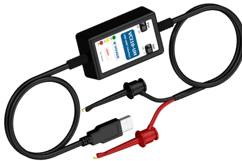
FIGURE 10. USB-HART communication interface [16]
