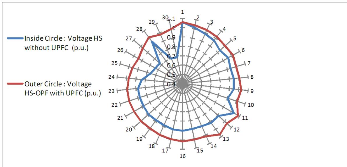
FIGURE 5. Comparison of bus voltages for 30 bus system using HS-OPF without and with UPFC
