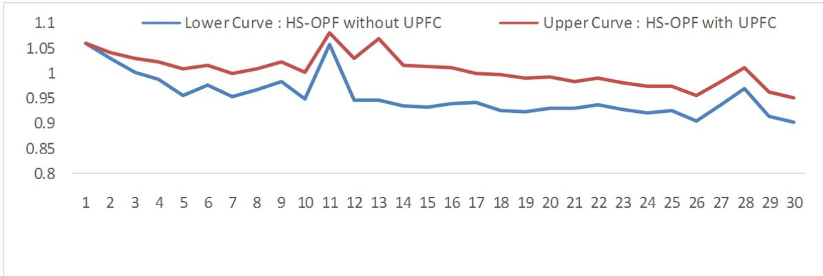
FIGURE 4. Comparison of voltage magnitude of optimal power flow without and with UPFC
