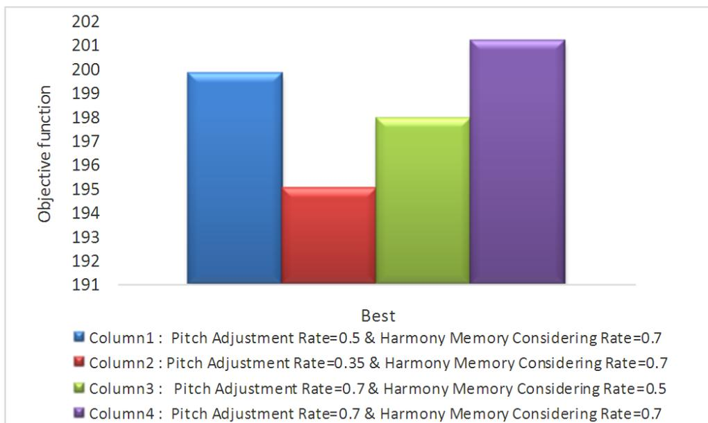
FIGURE 3. Multi-objective function value with change in HS algorithm parameters: PAR – pitch adjustment rate & HMCR – harmony memory considering rate
