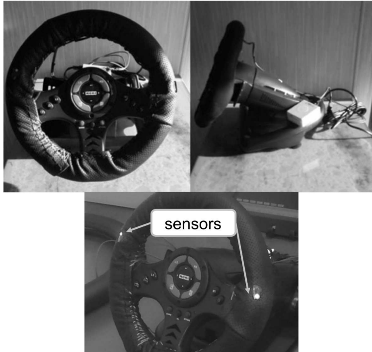
FIGURE 1. Appearance of the developed system. Sensors that can detect and measure the driver’s blood pressure are attached at positions of 10 and 2 o’clock on the wheel.
