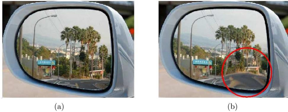
FIGURE 1. Curved mirror images of vehicles with reflection of street scene: (a) a flawless image; (b) a flawed image with distortion
