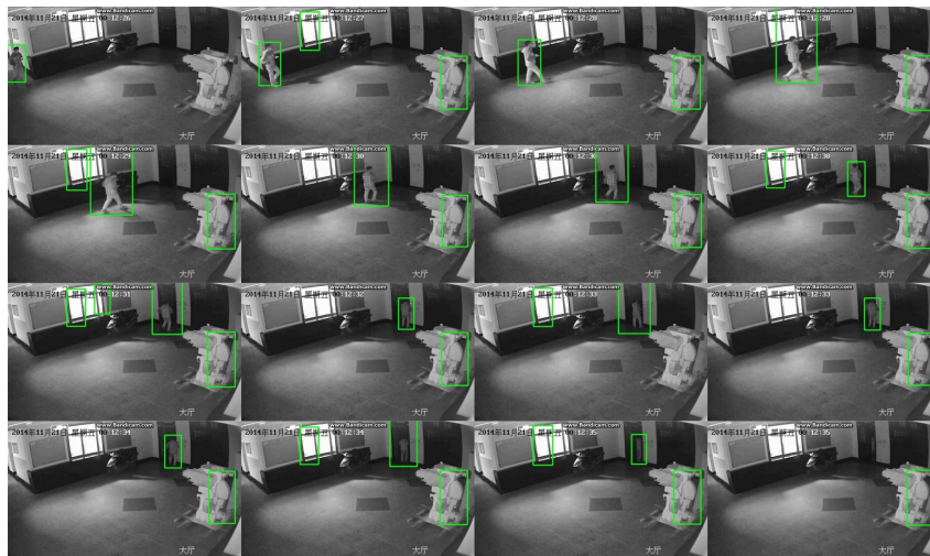
FIGURE 7. The detection results of the first video scene by using HOG+SVM algorithm
