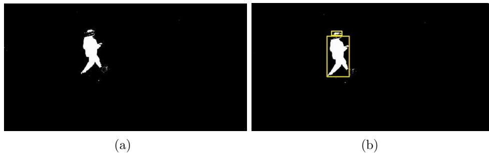
FIGURE 5. The 4-neighborhood searching algorithm: (a) foreground extraction; (b) the 4-neighborhood searching result
