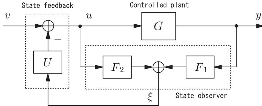
FIGURE 1. Configuration of control system
