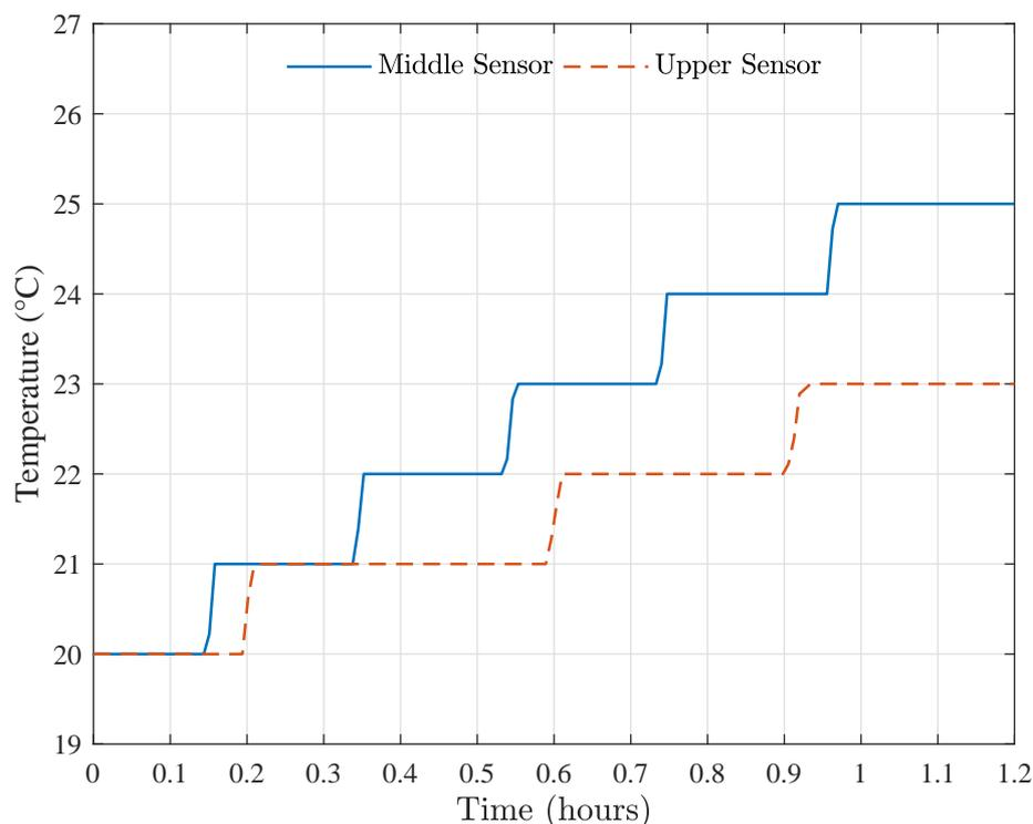
FIGURE 8. Thermal behavior of battery bank under 1C discharge
