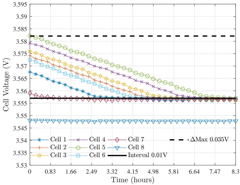
(a) Voltage of the equalization process (case 1)
