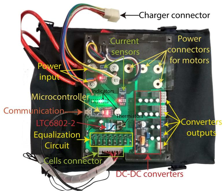
FIGURE 4. Prototype of the energy management system
