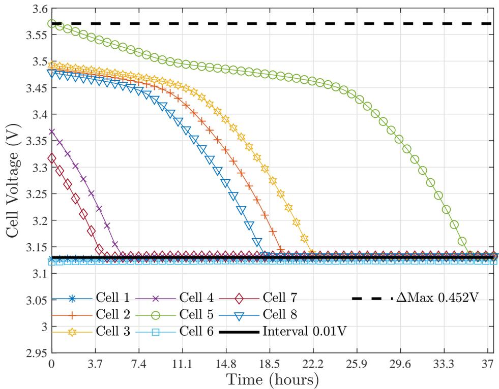
(b) Voltage of the equalization process (case 2)
