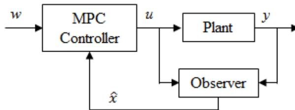
FIGURE 1. The structure of sequential MPC
