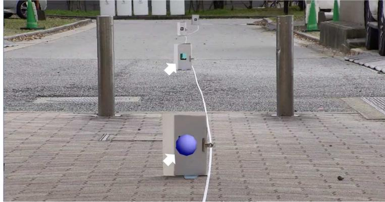
FIGURE 13. Marker detection with zoom magnification of 5x. Markers inside Zone 1 were successfully detected. The white arrows indicate the locations of the AR objects.
