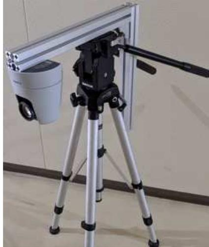
FIGURE 8. Camera system mounted on an aluminum frame with a tripod
