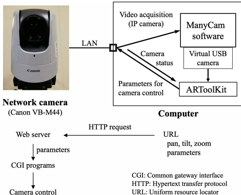
FIGURE 1. Combining a network camera with an AR environment using ARToolKit
