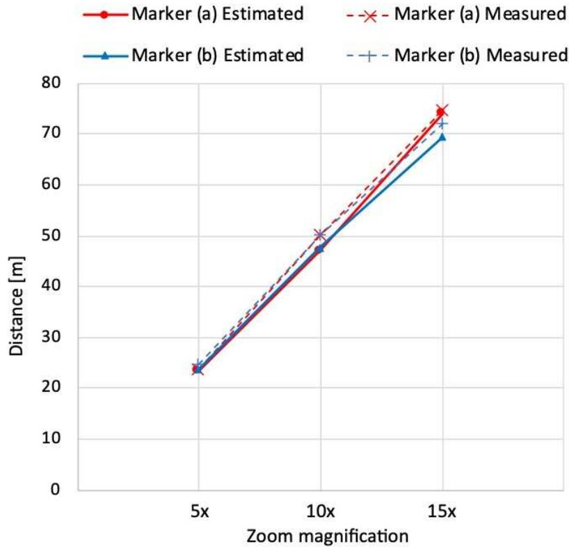
FIGURE 10. Applicable maximum distances between the camera and the marker for obtaining zone boundaries. The distance estimated by the distance-measurement function of ARToolKit and the distance measured using the laser range finder are shown for each background image shown in Figure 9 and each zoom magnification, that is, 5x, 10x, and 15x.
