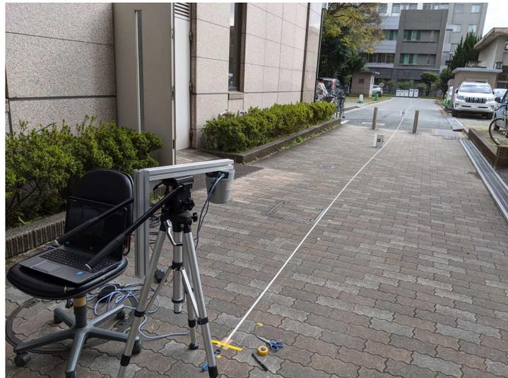
FIGURE 12. Experimental setup for zoning experiment. Markers are aligned in the depth direction from the AR camera system.
