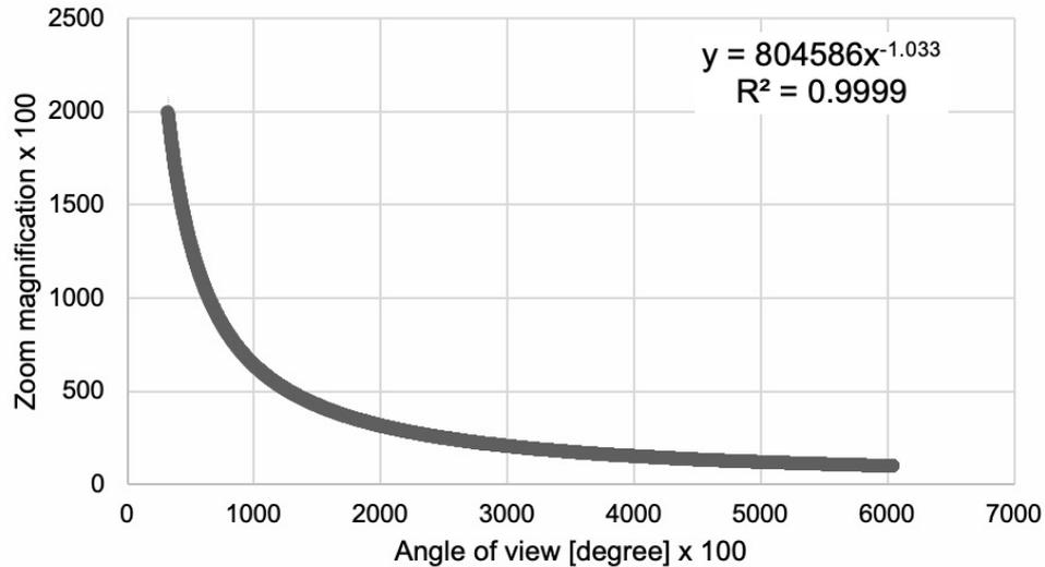
FIGURE 2. Relationship between zoom magnification and angle of view of the network camera. The vertical and horizontal axes correspond to a zoom-related parameter and angle of view-related parameter, respectively.
