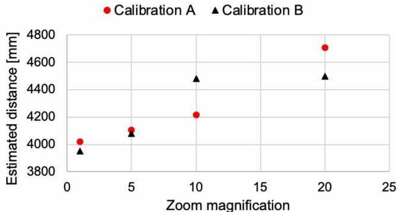
FIGURE 7. Comparison between the estimated distances averaged over three days for Calibration A and Calibration B
