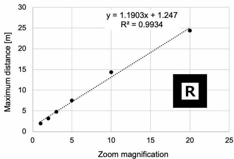
FIGURE 5. Maximum distances between the camera and the marker corresponding to the zoom magnifications when a square marker with a side length of 2 cm was used
