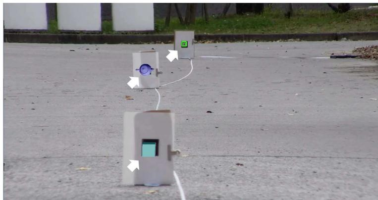
FIGURE 14. Marker detection with zoom magnification of 15x. Markers, including the farthest one in Zone 3, were successfully detected. The white arrows indicate the locations of the AR objects.
