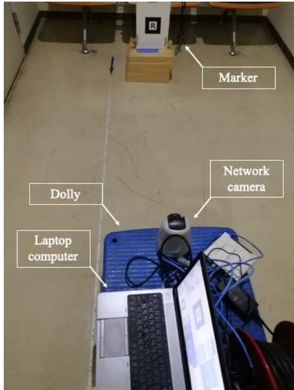
FIGURE 4. Network camera system with the laptop computer on a dolly
