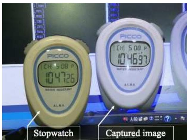
FIGURE 3. Snapshot of a stopwatch (left) and its displayed image (right) on the computer screen via the developed AR camera system
