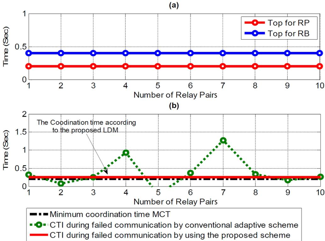
FIGURE 9. (a) The operation time for all pairs, and (b) the coordination time for all pairs, based on the proposed LDM scheme
