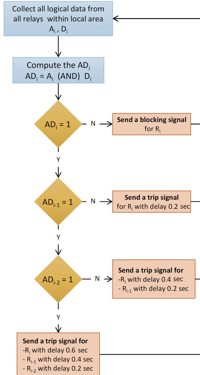
FIGURE 4. Flow diagram of the proposed LDM
