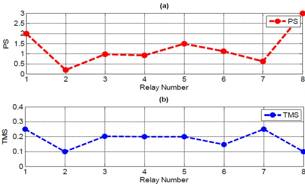
FIGURE 10. (a) Plug setting PS, and (b) TMS for all relays, by proposed scheme after the communication link return to the service
