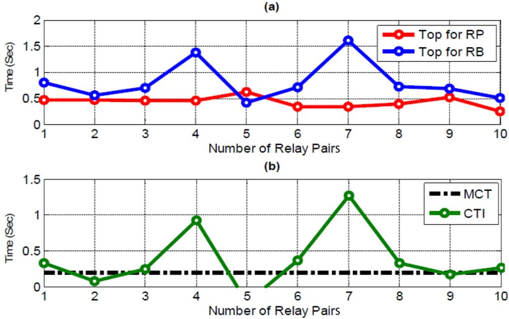
FIGURE 8. Communication link failure: (a) the operating time for all relay pairs after DG2 is integrated; (b) the coordination between primary and backup protection
