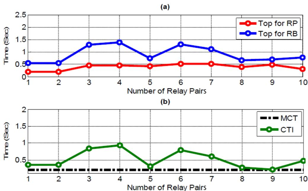
FIGURE 11. (a) Operating time relay pairs and (b) CTI and MCT for all for all relay pairs, by using optimal setting form the proposed scheme
