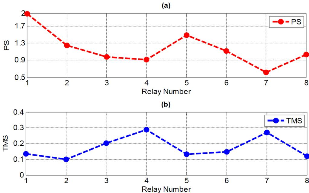
FIGURE 6. Relay setting from WAP center for all relays (a) Plug setting PS (b) Time multiple setting TMS for all relays
