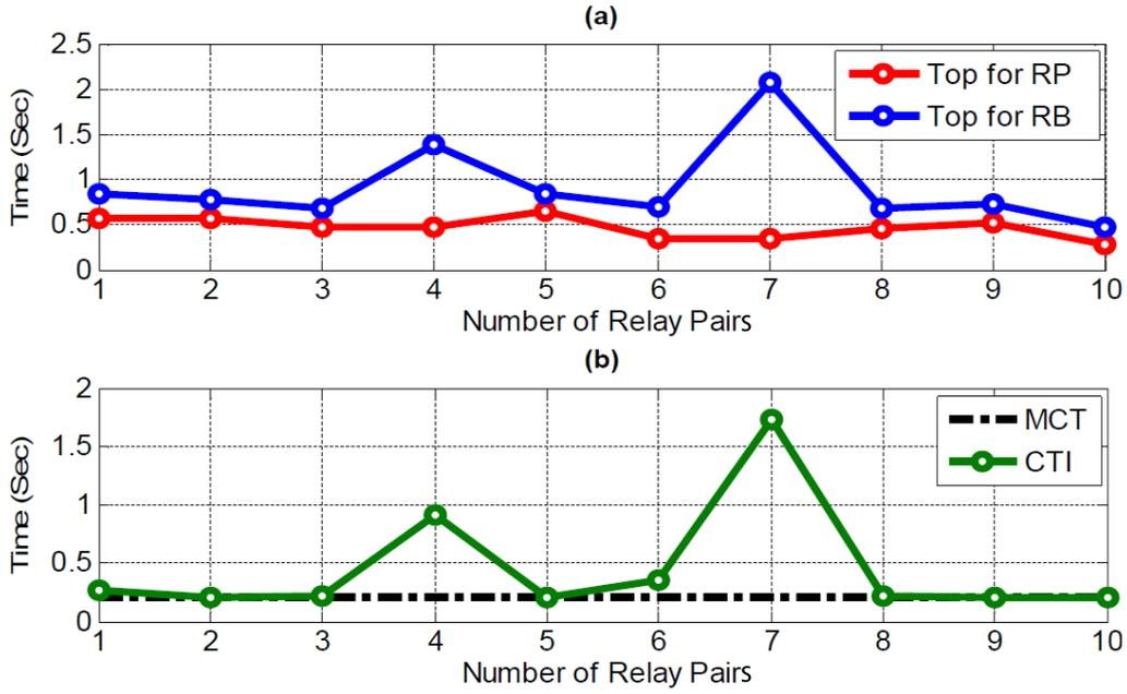
FIGURE 7. (a) Operating time in seconds for primary (RP) and backup (R-B) relays and (b) coordination time interval CTI and minimum coordination time MCT for all pairs of primary and backup relays
