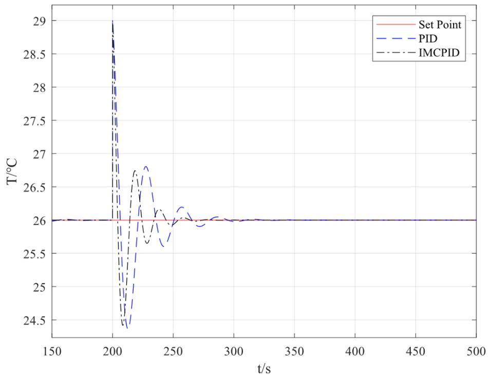
FIGURE 6. Interference curves of PID controller and IMCPID controller
