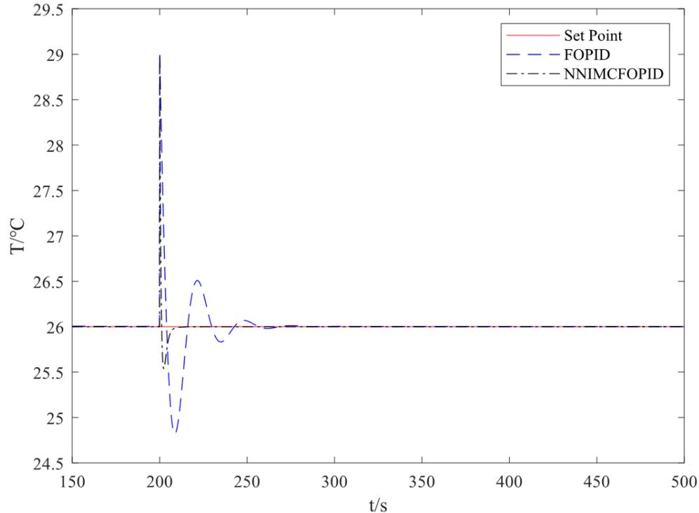
FIGURE 7. Interference curves of FOPID controller and NNIMCFOPID controller
