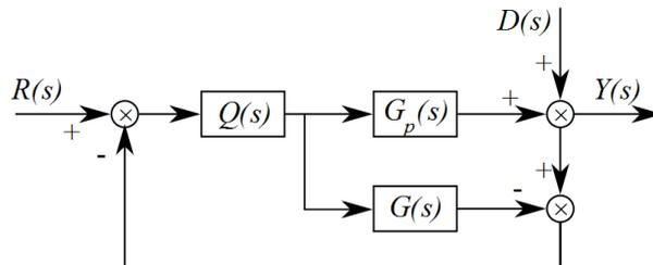
FIGURE 1. Block diagram of IMC system
