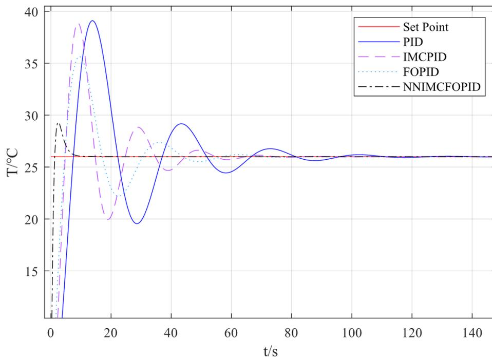
FIGURE 4. The response curve of each controller
