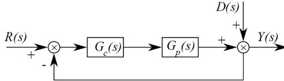
FIGURE 2. Equivalent feedback control structure
