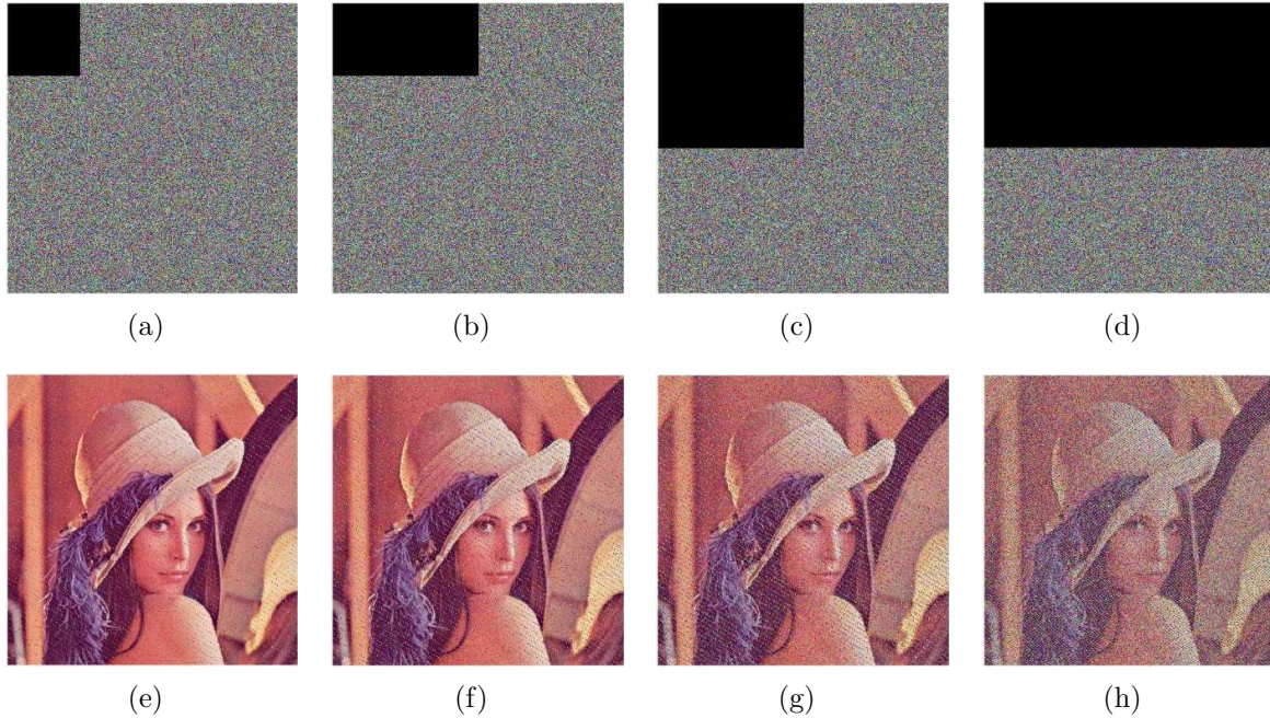
FIGURE 10. Simulation results of the tailoring attack: (a) cipher image (1/16 occlusion); (b) cipher image (1/8 occlusion); (c) cipher image (1/4 occlusion); (d) cipher image (1/2 occlusion); (e) recovered image (1/16 occlusion); (f) recovered image (1/8 occlusion); (g) recovered image (1/4 occlusion); (h) recovered image (1/2 occlusion)
