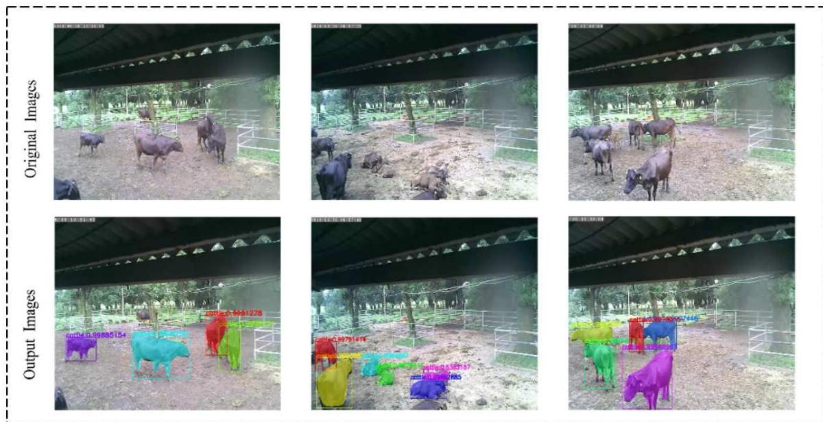
FIGURE 4. Cattle segmentation using the proposed Mask R-CNN
