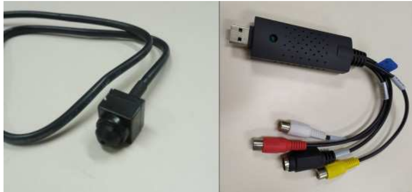
FIGURE 2. Analog camera and the analog-to-USB adapter used in this study
