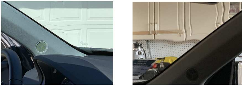
FIGURE 1. Two transmitted deformation scenes through defective car windscreens
