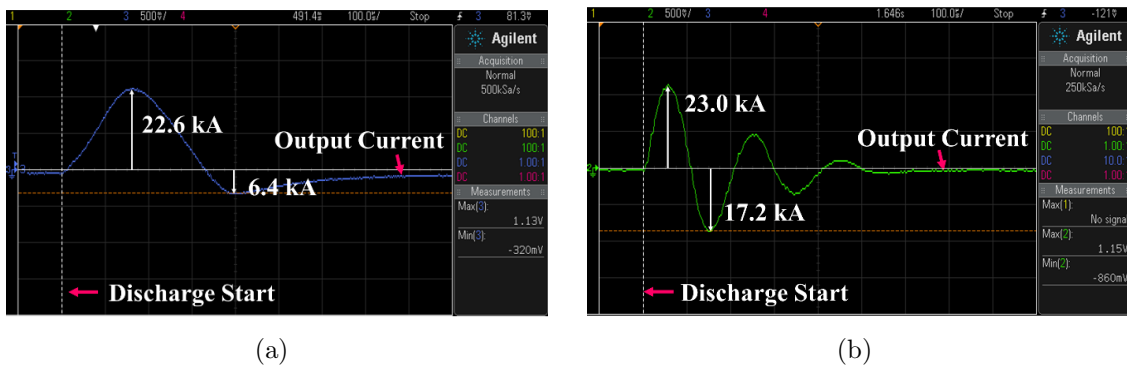
FIGURE 7. Measured output current of multipliers: (a) Proposed and (b) conventional [13]
