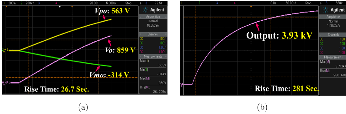
FIGURE 6. Measured output voltage of multipliers: (a) Proposed and (b) conventional [11]
