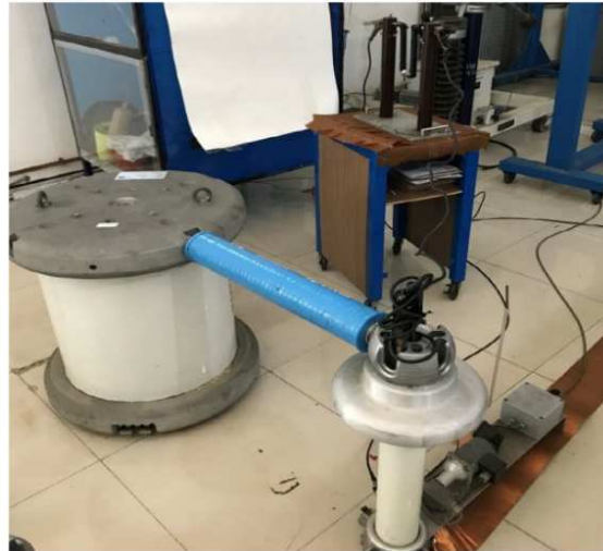
FIGURE 6. Test setup using test transformers
