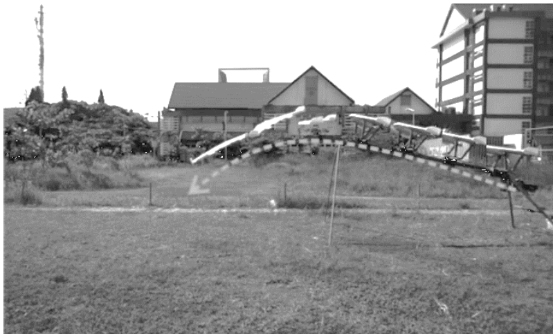
FIGURE 6. The UAV dummy executed takeoff with SET1 tension (20 kg)
