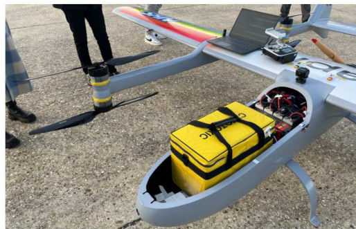
FIGURE 3. VTOL fixed-wing UAV (a 5 m wingspan) used for diagnostic samples delivery in Solen region, UK [24]
