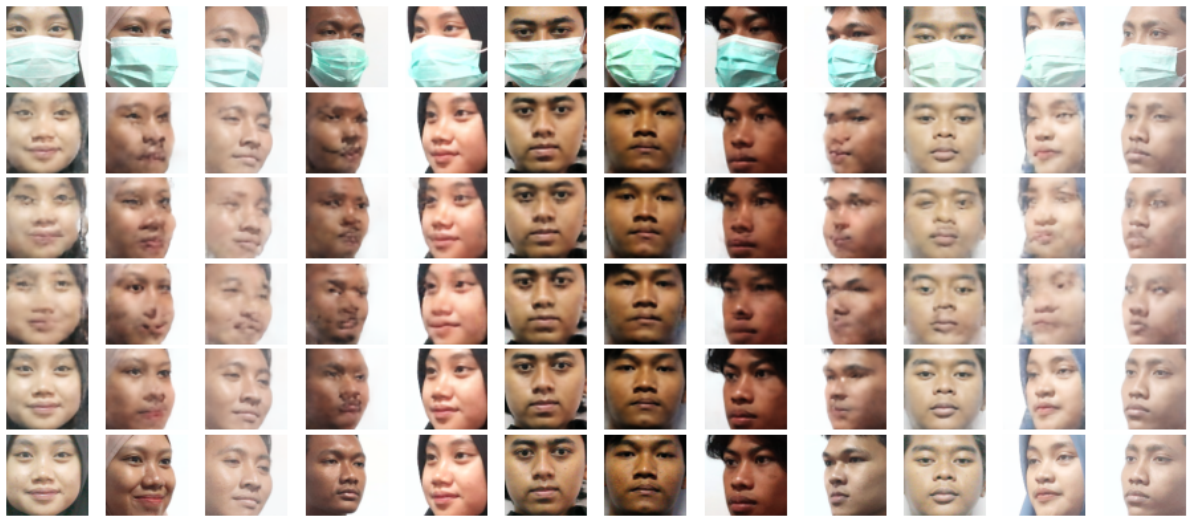
FIGURE 10. Result of the reconstruction model. The first row is the input images (a face with a mask), the second row is the reconstruction from the original U-Net, the third row is the reconstruction images from the U-Net with inception, the fourth row is the reconstruction from the V-Net with frozen pre-trained weights, the fifth row is the reconstruction from V-Net with unfrozen pre-trained weights, and the final row is the target images.
