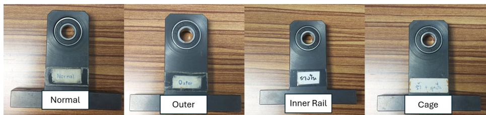
FIGURE 2. Bearing conditions used in the experiment
