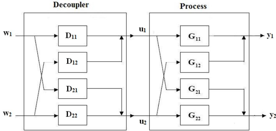
FIGURE 2. Architecture of system with decoupler
