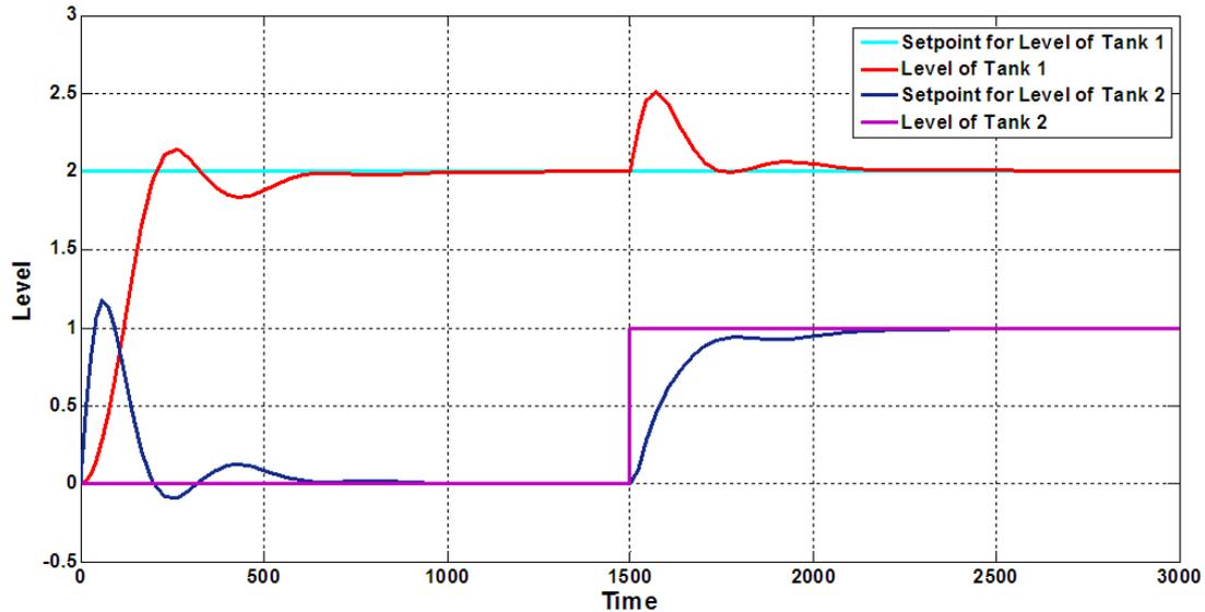
FIGURE 10. Response of PI controller in non minimum phase
