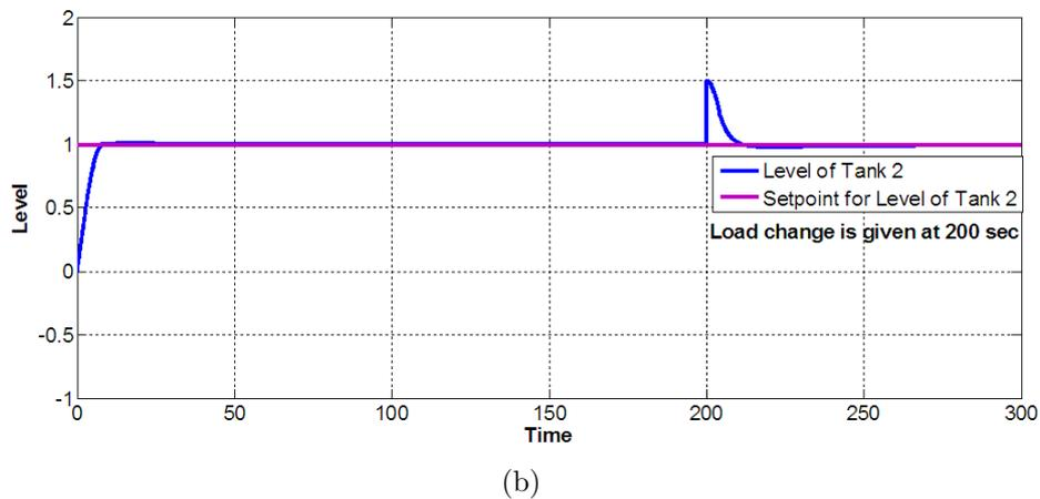
FIGURE 13. (a) Response of the PSO tuned PI controller for Tank level '1' in non minimum phase. (b) Response of PSO tuned PI controller for Tank level '2' in non minimum phase.
