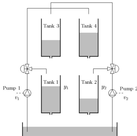
FIGURE 1. Schematic of quadruple tank system
