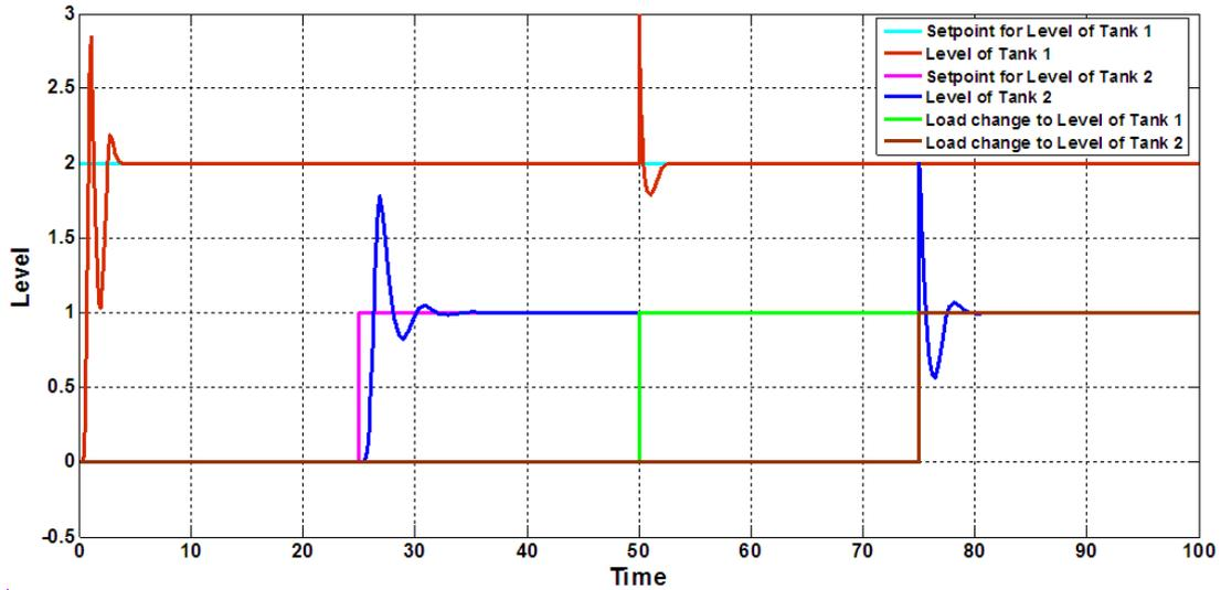
FIGURE 8. Response of PI controller with MRAC in minimum phase
