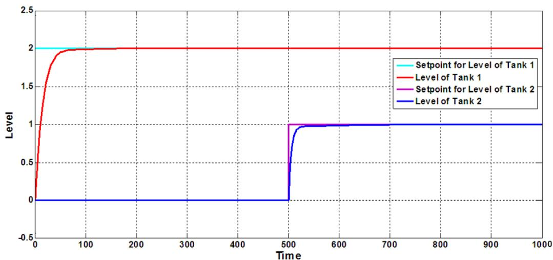
FIGURE 7. Response of PI controller with decoupler in minimum phase
