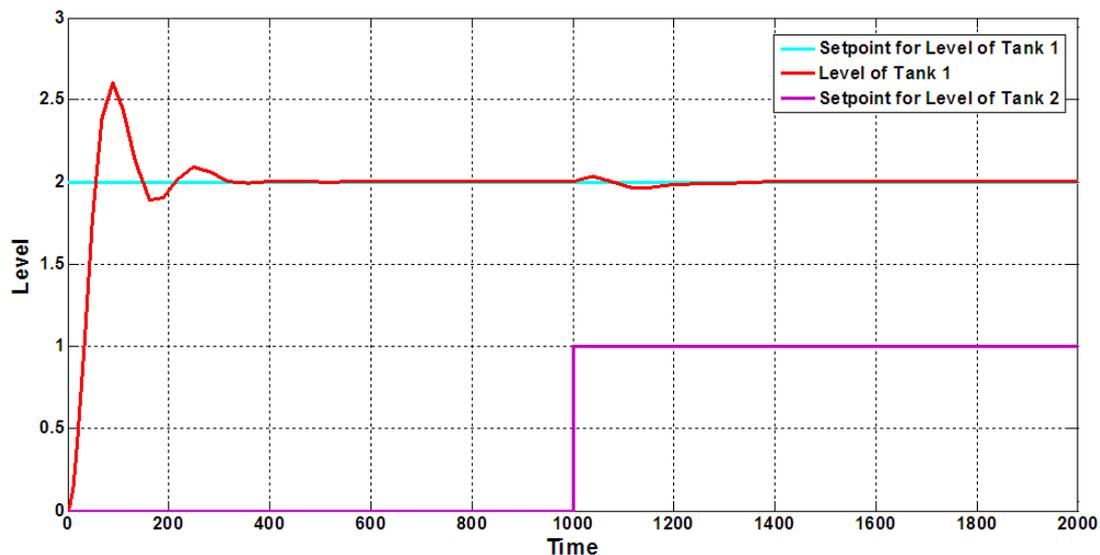
FIGURE 11. Response of PI controller with decoupler in non minimum phase
