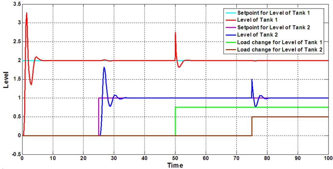
FIGURE 12. Response of the PI controller with MRAC in non minimum phase
