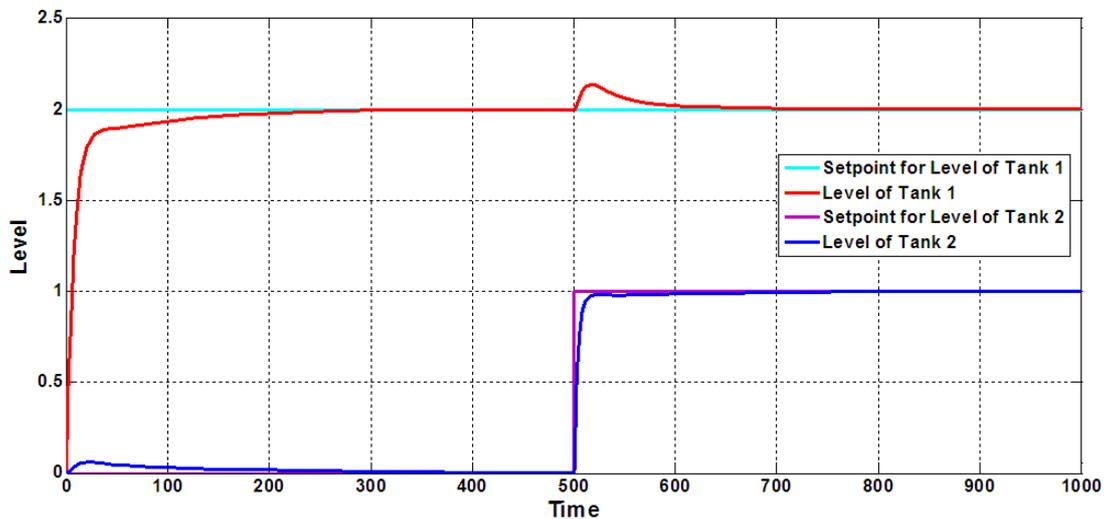
FIGURE 6. Response of PI controller in minimum phase
