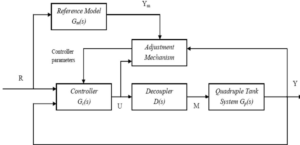
FIGURE 3. Structure of MRAC based control system for QTS
