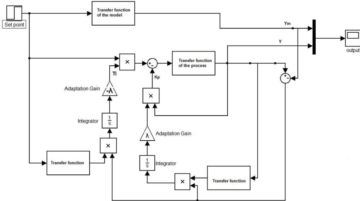
FIGURE 4. Adaptation mechanism for a single control loop using MRAC
