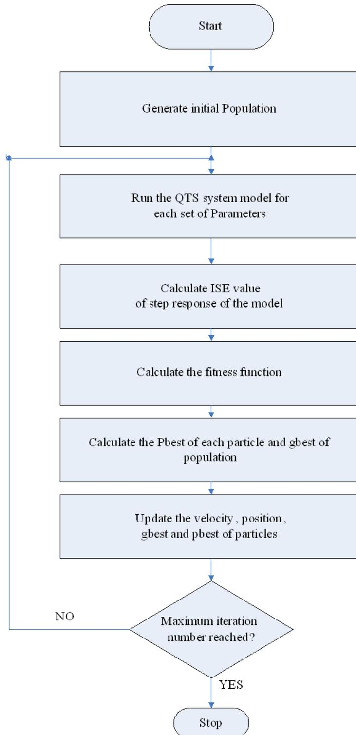
FIGURE 5. Flow chart for PSO algorithm
