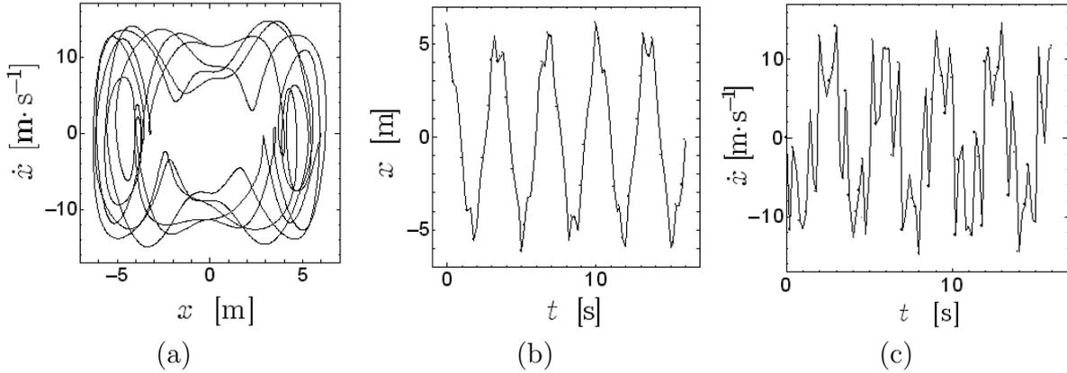
FIGURE 1. Oscillation and phase plane portrait of nonlinear systems of Van der Pol-Mathieu type: (a) phase plane portrait, (b) time evolution of  $x$ , (c) time evolution of  $\dot{x}$ ,  $\beta = 0.07875$  [s<sup>-1</sup>],  $\delta = 0.01$  [m<sup>-2</sup> · s<sup>-1</sup>],  $\gamma = 0.01$  [m<sup>-2</sup> · s<sup>-2</sup>],  $\omega = 10.0$  [rad · s<sup>-1</sup>],  $\mu = 20.0$  [s<sup>-2</sup>]
